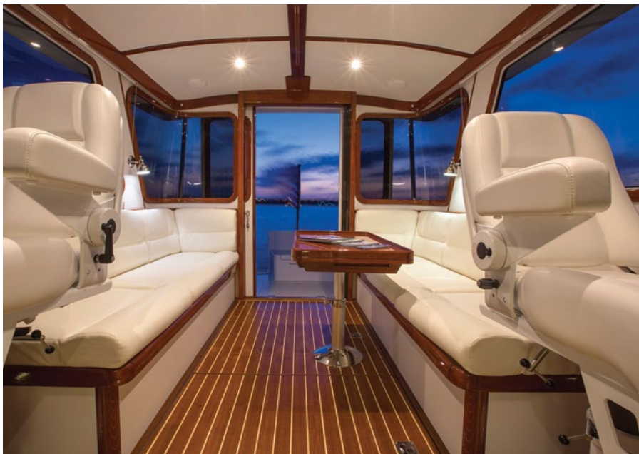
Except for the veneered sole, all the wood in the saloon is precisely joined mahogany.
