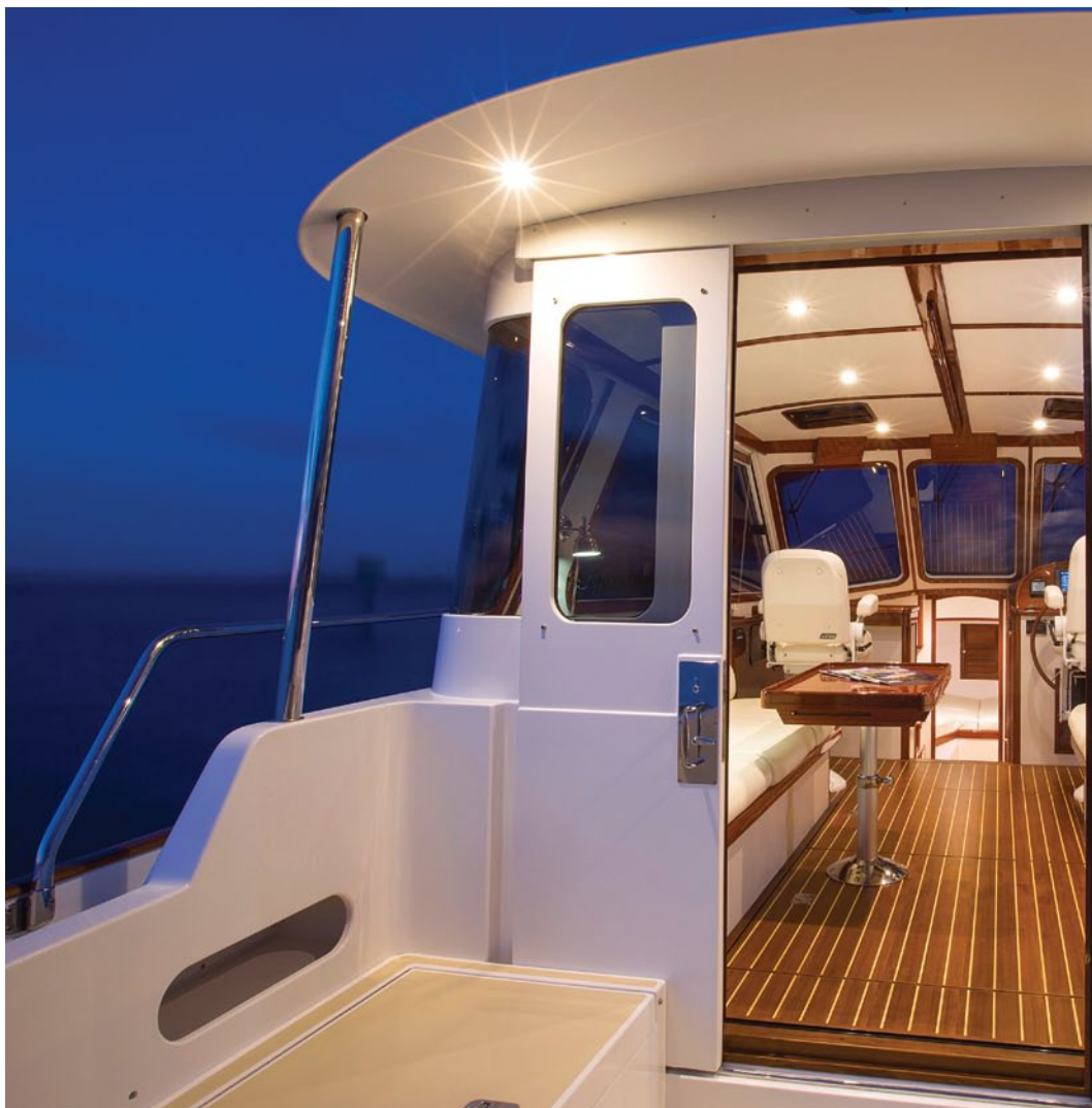
Except for the veneered sole, all the wood in the saloon is precisely joined mahogany.
